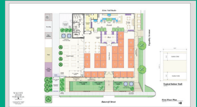
The floor plan shows fresh and dry market areas, stalls and dining spaces all wrapped by gardens at the front and a stage to one side.
